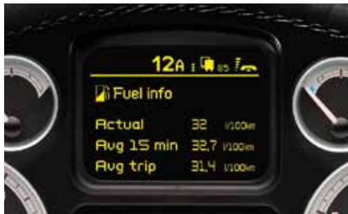
Actual and targeted fuel consumption is given on the display in the instrument panel.
