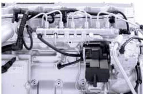
High-pressure commonrail injection, for powerful and economical engines.
