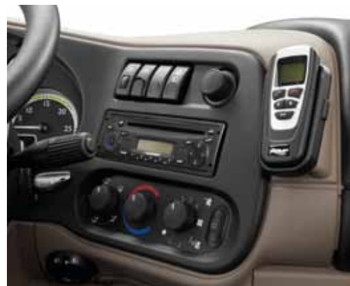
Optional dash-mounted position for mobile phone, pre-wired for 'hands free' connection with most GSM phones and steering wheel controls.
