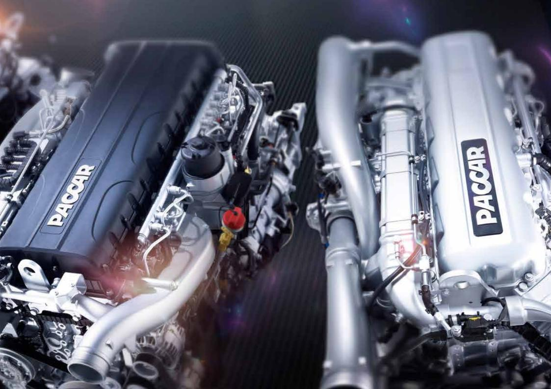
DAF developed for the new XF and CF the new 12.9 litre PACCAR MX-13 engine. Thanks to ultra modern and thoroughly proven technologies such as common rail injection, a variable-geometry turbocharger, exhaust-gas recirculation and ingenious exhaust-gas aftertreatment, the stringent Euro 6 emission requirements are met. At the same time, the six-cylinder PACCAR MX-13 engine is synonymous with maximum efficiency, high performance and low operating costs.
