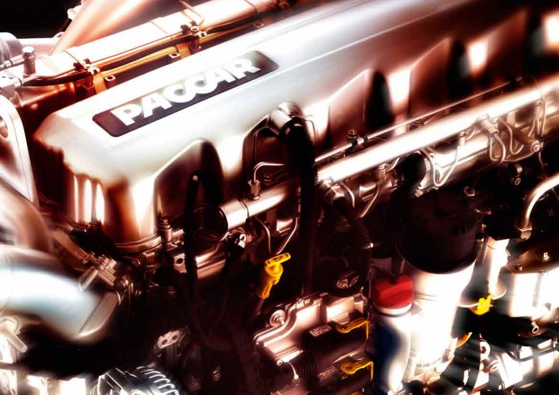
The new XF is powered by the new 12.9 litre PACCAR MX-13 engine. Thanks to ultra modern and thoroughly proven technologies such as common rail injection, a variable-geometry turbocharger, exhaust-gas recirculation and ingenious exhaust-gas aftertreatment, the stringent Euro 6 emission requirements are met. At the same time, the PACCAR MX-13 engine is synonymous with maximum efficiency, high performance and low operating costs.
