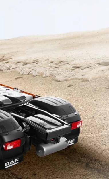
**SPACE** One of the starting points in developing the chassis was to create as much space as possible. The SCR catalytic converter and particulate filter are combined in one unit. The AdBlue tank is positioned practically under the cab. The result: all the space for pump installations or hydraulic tanks, or fuel tanks with volumes up to 1,500 litres.
