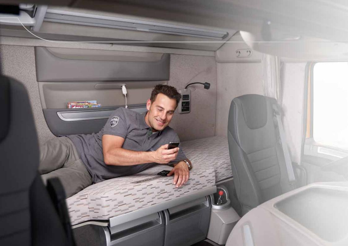
**SPACIOUS** The new XF offers an abundance of space. The work and living space of 12.6 m<sup>3</sup> and standing hight of 2.25 m in the Super Space Cab are unequalled. The storage space is also market leading. No less than 675 litres under the bed, with space for a fridge in which even large bottles can stand upright.
